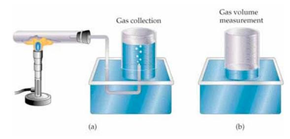
Gas is collected over water so that the atmosphere is not present. Water levels made equal so pressure inside is equal to that outside
